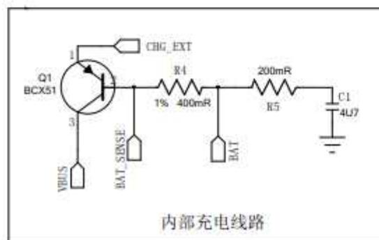
Note: the use of internal charging current up to 250mA.
